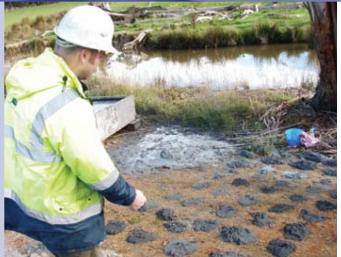
Bore logging of geological layers (above) is an important aspect of data collection in the resource appraisal process.
